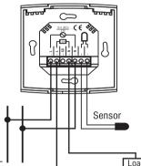
Do not place the floor sensor directly next to an ele- L N ment but rather for maximum performance, the floor sensor should be centred between the wires in mat (80°C max.). The temperature sensor wire can-
